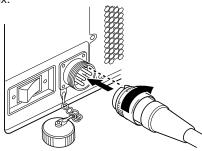
2 Insert the plug of the supplied power cord into a wall outlet, and turn the plug to right to fix.
